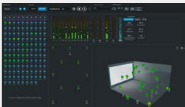
Dolby Atmos Renderer application. The top right yellow box highlights the speaker control section, and the top left yellow box indicates the available speaker layout selections.
