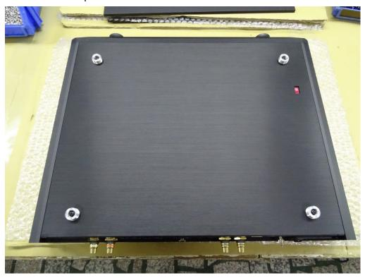
Remove the screws in the red frame for a total of 6 pieces to remove the EVO DAC cover.
